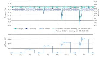
Figure 9: Transient behavior with HVO fuel
